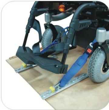
Fitting the front restraint
