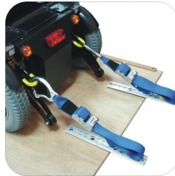
Fitting the rear restraint
