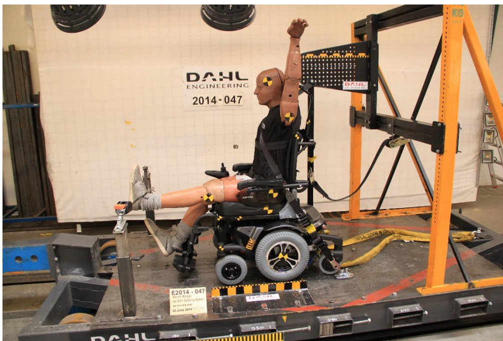
Leon crash test using Dahl Docking station.
