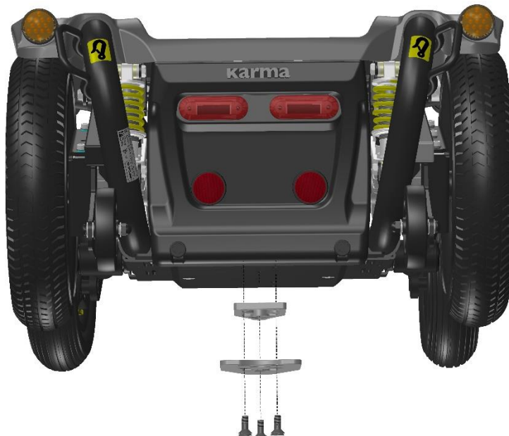
mounting the Dahl docking plate on to the Leon chassis
