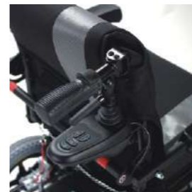
The optional quick release steering controller enables maneuvering switches from the user to the attendants in seconds.
