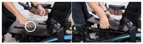
Step 4: Use 4 mm Allen key to unscrew the bolt connecting the seat plate to take off the seat plate. When taking off the seat plate, first tilt it up and then pull.
