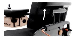
Step 2: Adjust the armrest to the proper height and re-tighten the bolts. Now the armrests are set in to a different height position.
