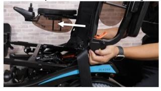
Step 5: Push the backrest frame to the preferred position. If the frame is tight, use rubber mallet to help.
