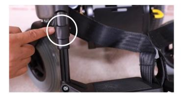
Use 10 mm open wrench and 5 mm Allen Key from KARMA Tool Kit to loosen the bolt at the side of the footplate and adjust the footplate height and retighten the bolt. Now the footplates are set in to a different position.
