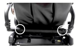
Step 1: Use 5 mm Allen key to unscrew the screws securing the armrests.
