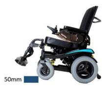
Driving down of a higher surface (like pavement), always be aware of the sudden forward movement of your wheelchair when driving down of it. If your wheelchair has powered seat tilt, you can use the seat tilt for more stability whilst driving of the pavement.
