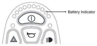
If the maintenance free batteries are fully charged, all ten LED's on the top bar light up. The more energy is used the more LED extinguish, starting on the right side.
