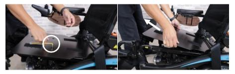
Step 2: Use 4 mm Allen key to unscrew the bolt connecting the seat plate. When taking off the seat plate, first tilt it up and then pull.
