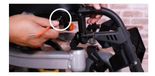
Step 1: Use 5 mm Allen Key included in your KARMA Tool Kit to remove the screws under the seat.
