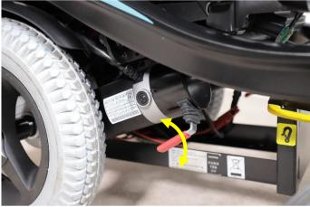
Testing the brake release
