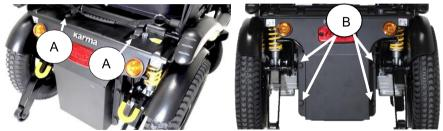
After taking the cover off, the maintenance free battery can be pulled out of the box. Mind the cables! At installing the maintenance free battery, one should pay great attention to make sure the cables are not jammed between the battery and the battery box.
