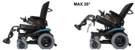
If the tilt is activated over a certain angle, the driving speed will be reduced. This is to reduce the risk of danger whilst driving at high speed.
