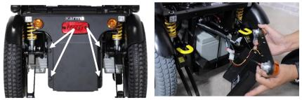
Step 7: Untighten these 4 knobs on the both sides to take off back-rear cover.
