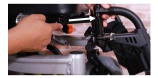
Step 2: Pull out or push in the footrest hanger and find the mounting hole that best fitted the user.
