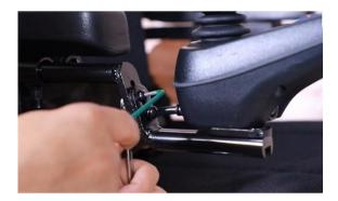
Step 1: Use 3 mm Allen key and 8 mm open wrench to loosen up this bolt.
