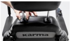
Adjust the height of the headrest from this button under the headrest.
