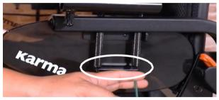
Step 1: Use 3 mm Allen key to remove two screws shown above.
