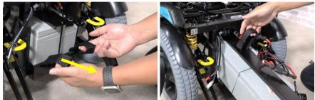
Step 9: Use the rear and front strap to pull out the battery plate.
