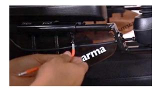
Step 1: Use 5 mm Allen key to loosen up this bolt.
