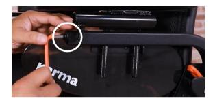
Step 2: Use 5 mm Allen key to remove the screw shown above.
