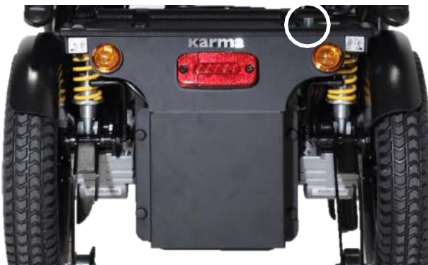
Circuit breaker location
