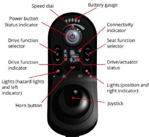
Control Panel with No Tilt & Lighting System
