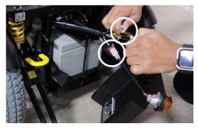
step 8. Disconnect the two light cables
