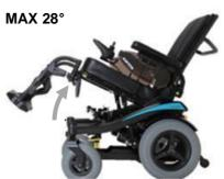
If the tilt is activated over a certain angle, the driving speed will be reduced. This is to reduce the risk of danger whilst driving at high speed.
