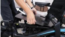
step 2. Use 4mm Allen key to unscrew the bolt connecting the seat plate. When taking off the seat plate, first tilt it up and then pull.
