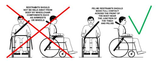
Picture of improper belt fit
