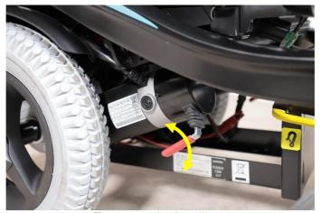
Testing the brake release
