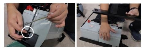
step10. Use 8mm open wrench to loosen up this bolt.
