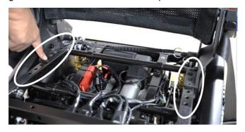
step 4. Use 5mm Allen key to unscrew the bolts connecting the frame.
