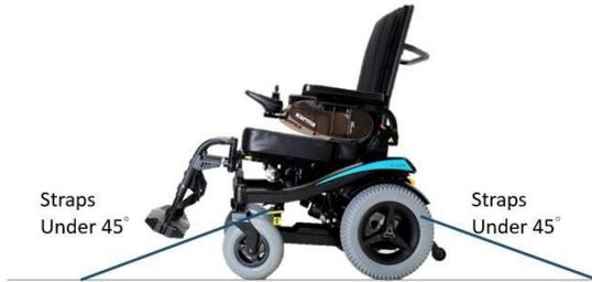
The angle of the straps should be around  $45^\circ$  to the horizontal plane. This is to have maximum effect in vertical and horizontal direction.
