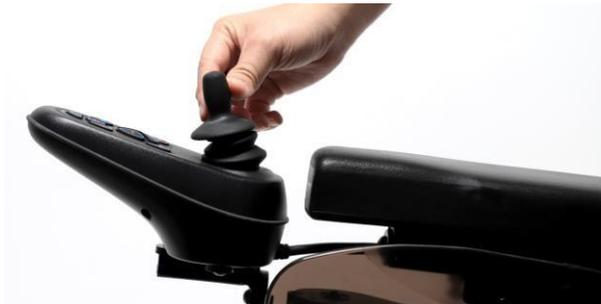
Step2. Push the joystick forwards until the control system beeps.
