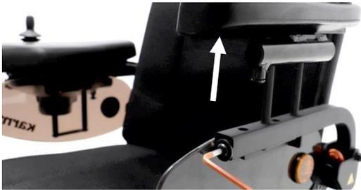
step 2: Adjust the armrest to the proper height and re-tighten the bolts. Now the armrests are set in to a different height position.
