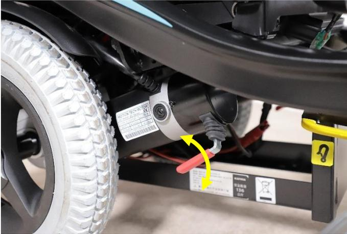
*Testing the brake release*
