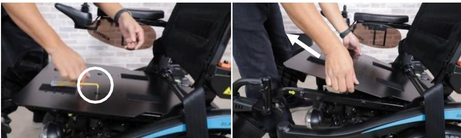
step 2. Use 4mm Allen key to unscrew the bolt connecting the seat plate.
