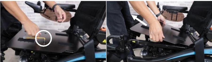
step 4. Use 4mm Allen key to unscrew the bolt connecting the seat plate to take off the seat plate. When taking off the seat plate, first tilt it up and then pull.
