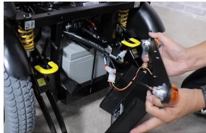
step 7. Untighten these 4 knobs on the both sides to take off back-rear cover.
