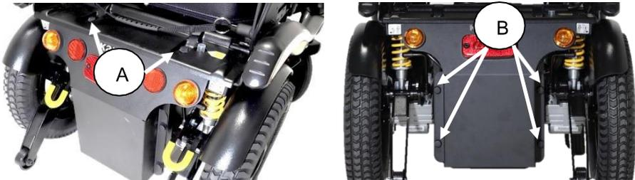
After taking the cover off, the maintenance free battery can be pulled out of the box. Mind the cables! At installing the maintenance free battery, one should pay great attention to make sure the cables are not jammed between the battery and the battery box.
