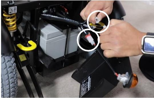
step 8. Disconnect the two light cables
