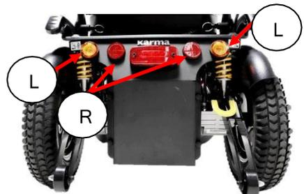
The chassis has very strong and bright LED lights to make sure you can have a safe drive in the dark. The optional orange reflectors and the red reflectors can also make you visible for other people as well. The lights fulfill the European requirements. The additional LED indicators give our environment clear information in which direction you want to go.
