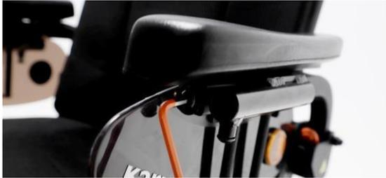
step 1: Use 5mm Allen Key from KARMA Tool Kit to loosen the heightadjustment bolts under the armrest pad.
