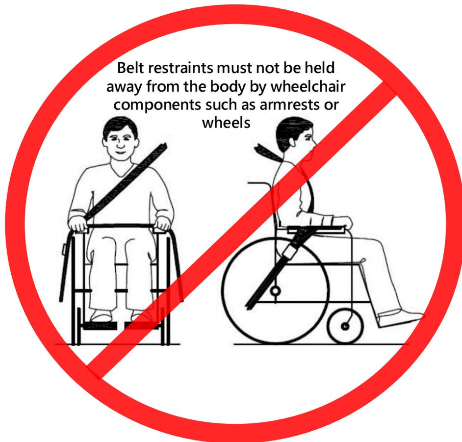
Illustration of improper belt-restraint fit
