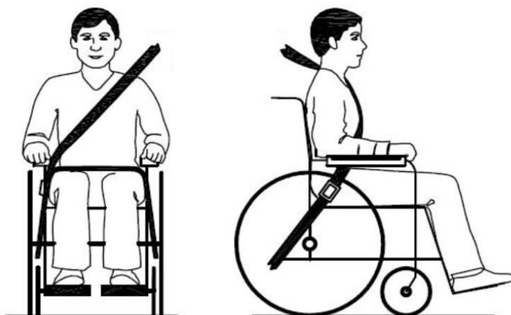
Illustration of proper belt-restraint fit
