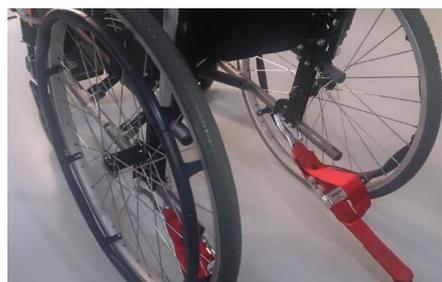
Fitting the Rear Restraint
