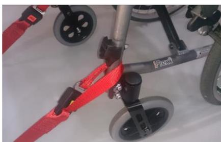
Fitting the Front Restraint
