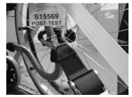
Fitting the rear restraint
