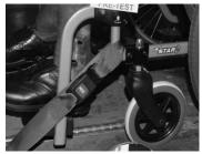
Fitting the front restraint
