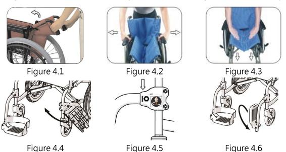
While completing step 2, never put your fingers around the sides or under the wheelchair as they can be trapped between the seat and the frame. (See the right figure.)
