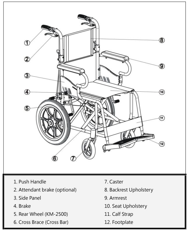
\* KM-2500L is equipped with 20" rear wheels.
