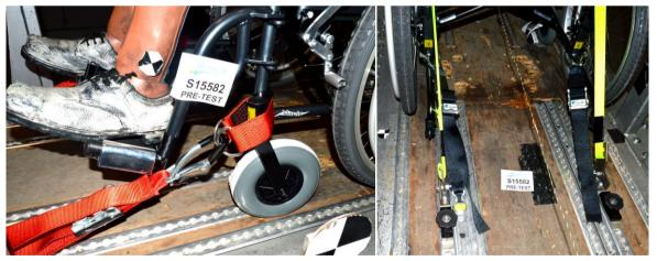
Fitting the Front Restraint
