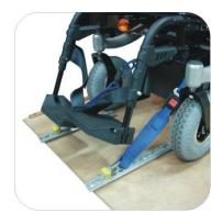
Fitting the front restraint
