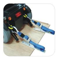
Fitting the rear restraint
