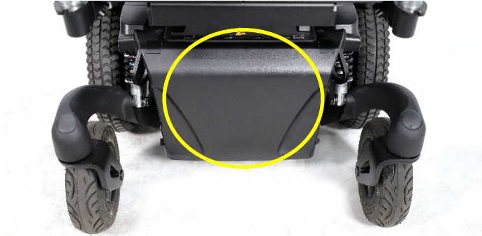
Position of the front maintenance free batteries
