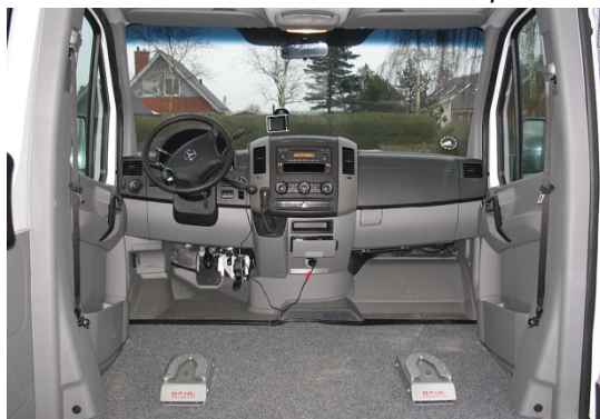
Dahl Docking Station mounted on the floor
