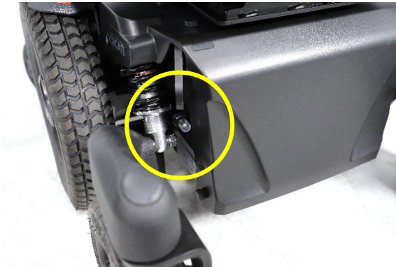
Position of the circuit breaker
