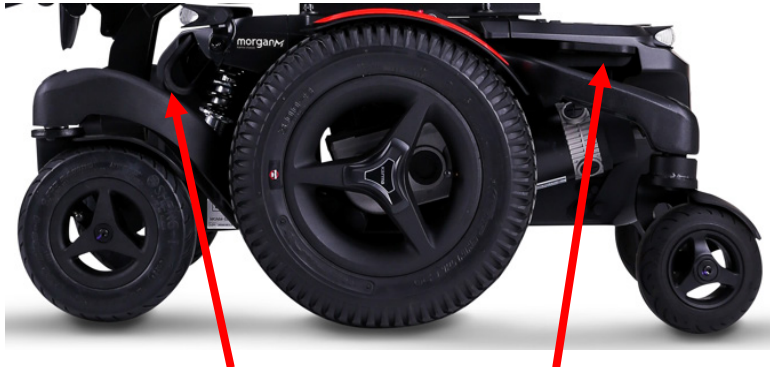
Fixation loops in the front Fixation loops in the rear
