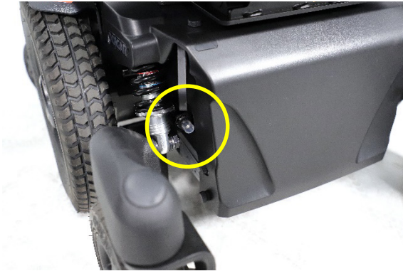
Position of circuit breaker
