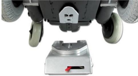
*Docking station and docking plate on chassis*
