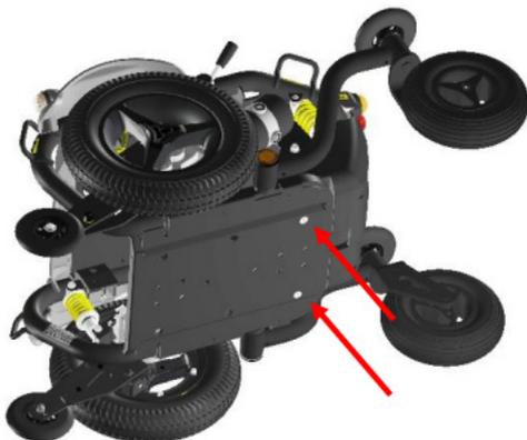
Step 6: Mount the Dahl locking plate by using the 5 high grade Dahl bolts on to the chassis. Secure them with Loctite 222 and tighten them, but not too tight. (16-18 Nm).
