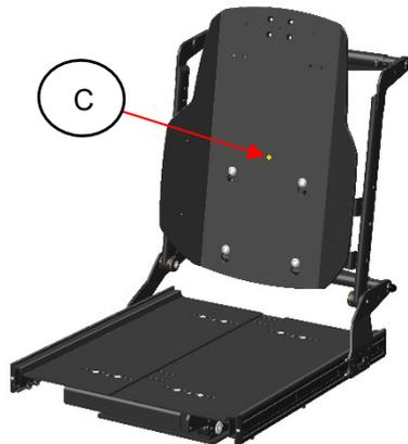
Step 3: Place the backrest panel into the backrest mounting frame and secure it by the lock bolt (C).
