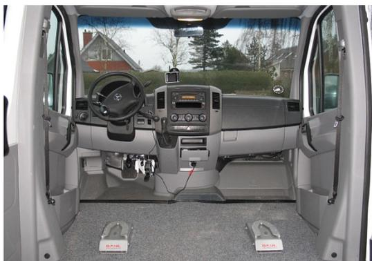
*Dahl docking station mounted on the floor*
