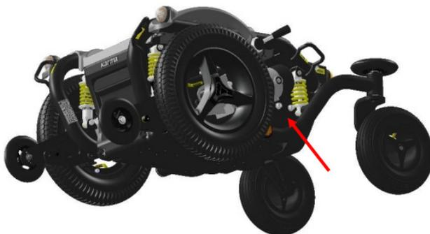
Step 3: Pull out the battery box and disconnect main battery cable.
