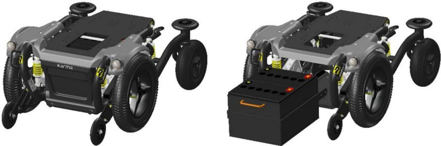
*Position of the front maintenance free batteries*
