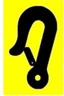
The wheelchair is designed to use a four-point heavy duty webbing restraint. For this matter the wheelchair has two brackets on the front end and two brackets on each rear side of the chassis. The brackets are indicated with a sticker. These anchoring points shall be used to connect the tie-down belt to.
