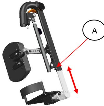
Step 1: Slowly loosen the legrest fixation bolt (A), using a 4 mm Allan key. Just enough to feel the footplate is starting to move.
