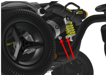
Step 11: Place the front cover back and secure it with the two bolts.
