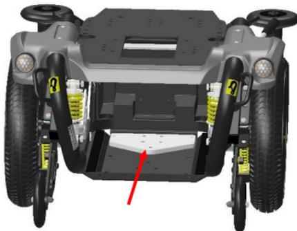
Step 5: Tighten the two bolts into the mounting holes to fix the mounting plate.
