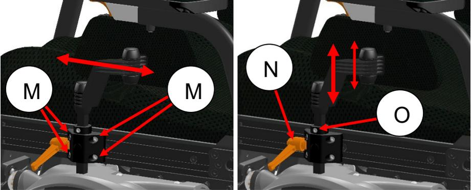
Step 1: Loosen the four bolts (M) using a 5 mm Allan Key.
