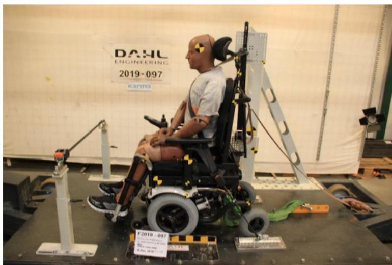
The locking of the wheelchair into the Dahl Docking station makes it much easier to lock down the wheelchair for occupied transportation. It can be used also for wheelchair users who want to drive the car by themselves.
