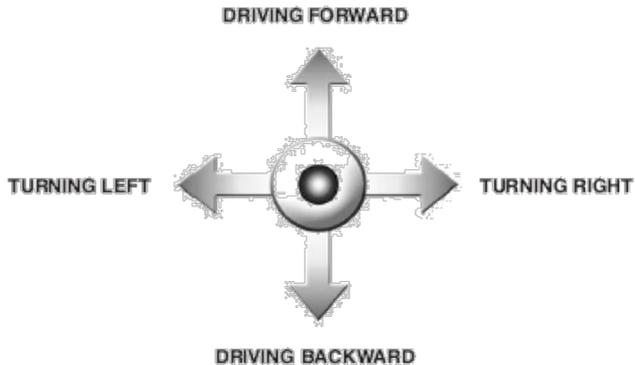
The secondary purpose of the joystick is to navigate through menu of the wheelchair. By moving the joystick forward or backward you can scroll up or down through the menu, by moving to the right you can enter a sub selection.
