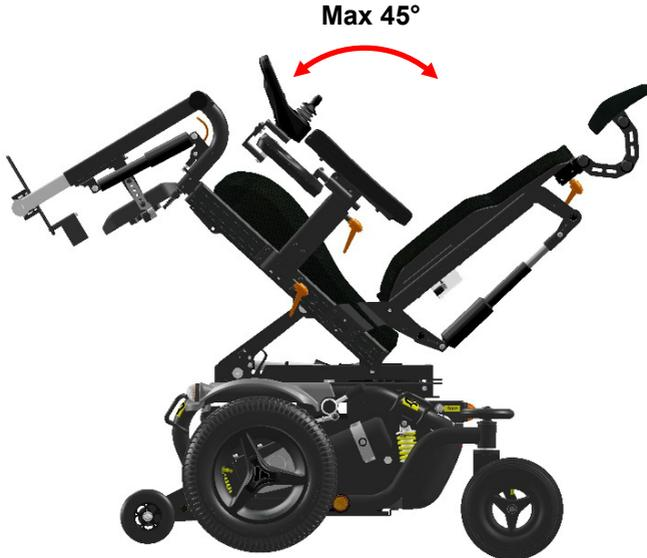
If the tilt is activated over a certain angle, the driving speed will be reduced. This is to reduce the risk of danger whilst driving at high speed.
