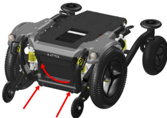
Step 2: Loosen the 4 locking bolts of the battery box.
