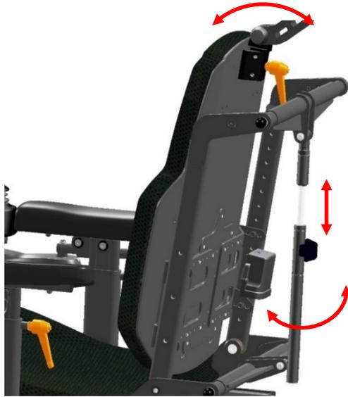
The mechanical adjustable recline backrest uses a stepless telescopic tube with quick release and lock lever action. The manual stepless recline backrest can be set up to 115°.
