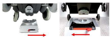
The release lever on the DAHL DOCKING STATION MK II (Left) and DAHL VARIODOCK™ (Right)
