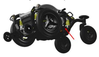
Step 3: Pull out the battery box and disconnect main battery cable.
