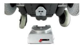
Docking station and docking plate on chassis
