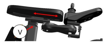
Step 1: Loosen the bolts (V) using a 5 mm Allan key.
