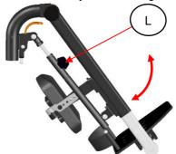
Step 1: To adjust and set the legrest angle, you hold the legrest with one hand and unlock the setting lever (L) with the other hand and push the legrest sideways.
