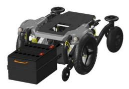
Step 4: Place the mounting plate inside the chassis on the bottom.
