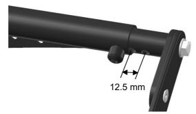
Step 5: Secure the right position by mounting the dome shaped bolts into the designated holes again, then tighten the end bolts to fix that side of the seat.
