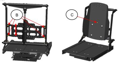
Step 3: Place the backrest panel into the backrest mounting frame and secure it by the lock bolt (C).
