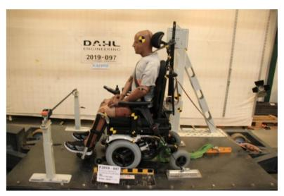
The locking of the wheelchair into the Dahl Docking station makes it much easier to lock down the wheelchair for occupied transportation. It can be used also for wheelchair users who want to drive the car by themselves.
