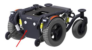
Position of the battery pole (behind the front cover)
