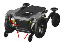
Step 2: Remove the four battery box locking bolts at the rear end of the chassis side.
