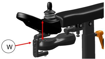
Step 1: Loosen the 2 bolts (W) using a 3 mm Allan key.
