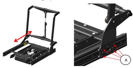
Step 1: Loosen the 4 bolts on each side of the backrest bracket (A) by using a 4 mm Allan key.
