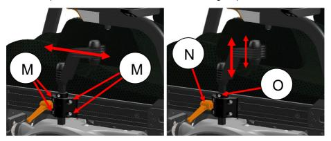
Step 1: Loosen the four bolts (M) using a 5 mm Allan Key.
