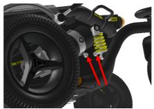
Step 3: Pull the battey box slowly out of ther chassis and mind the cables.
