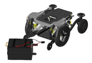
Step 5: Lift the batteries out of the box and disconnect the cables of the poles using a wrench.
