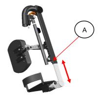
Step 1: Slowly loosen the legrest fixation bolt (A), using a 4 mm Allan key. Just enough to feel the footplate is starting to move.
