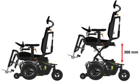
Whilst lifting the seat, the driving speed will always automatically be reduced to gain maximum stability. At high seating position also, the seat tilt will be blocked to gain maximum stability. The seat height can be set to every height position by the user.
