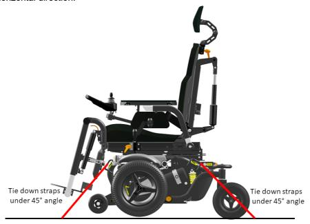
The straps have to be connected to the vehicle at suitable anchor points. Make sure that the tire pressure is at the recommended level so the straps can have maximum effect. Make sure the straps are tightened to maintain optimal security.
