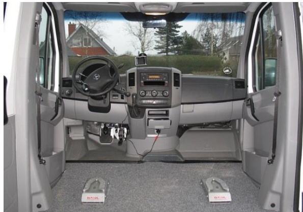
Dahl docking station mounted on the floor
