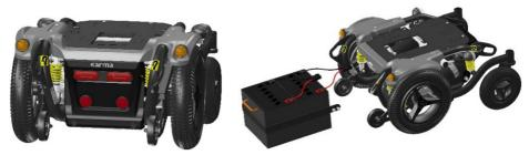
Position of the maintenance free batteries
