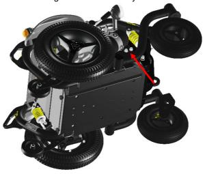
Step 3: Pull out the battery box and disconnect main battery cable.
