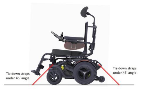
The straps have to be connected to the vehicle at suitable anchor points. Make sure that the tire pressure is at the recommended level so the straps can have maximum effect. Make sure the straps are tightened to maintain optimal security.
