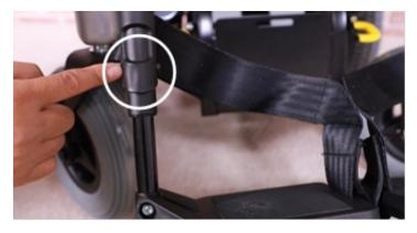
Step 2: Adjust the footplate height and re- tighten the bolt and nut. Now the footplates are set into a different position.
