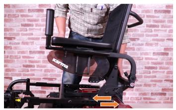
Adjust the seat depth according to the requirements, and then tighten them up (Required tools: 5 mm Allen key and #13 Open Wrench).
