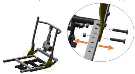
Step 4: Lift the seat and move it forward or backward to the desired position.
