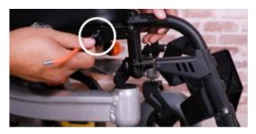
Step 2: Pull out or push in the footrest hanger and find the mounting hole that best fits the user
