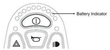
If the maintenance free batteries are fully charged, all ten LED's on the top bar light up. The more energy is used the more LED extinguish, starting on the right side.
