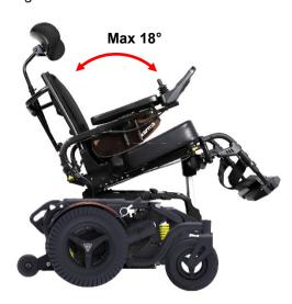
If the tilt is activated over a certain angle, the driving speed will be reduced. This is to reduce the risk of danger whilst driving at high speed.
