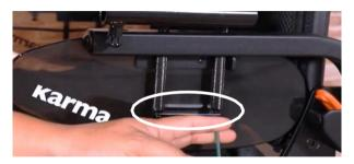
Step 2: Use 5 mm Allen key to loosen the height adjustment bolt shown above.
