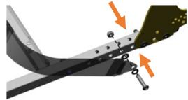
Step 5: Secure back the seat pan and put back the seat cushion.
