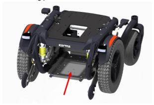
Step 5: Tighten the two bolts into the mounting holes to fix the mounting plate.
