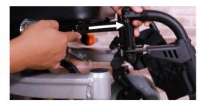
Step 3: Re-tighten the screws. Now the footrests are set into a different position.
