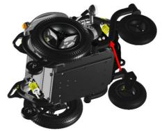
Step 3: Pull the battey box slowly out of ther chassis and mind the cables.
