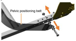
Step 3: Use a 5 mm Allen key and #13 Open Wrench to remove these 4 bolts and nuts connecting the backrest tube frame. There are holes for incremental adjustments which are in increments of 25.4 mm (1").
