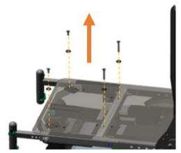
Step 2: Use a 5 mm Allen key and #13 Open Wrench to remove the pelvic positioning belt.
