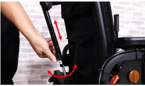
The mechanical adjustable recline backrest uses a stepless telescopic tube with quick release and lock lever action. The manual stepless recline can be set up to 119°.
