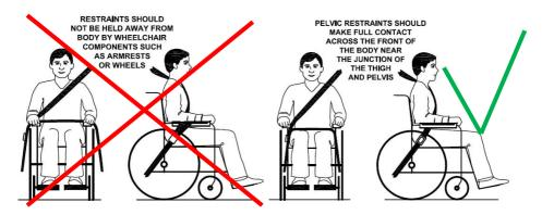
Picture of improper belt fit
