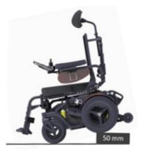
Driving down of a higher surface (like pavement), always be aware of the sudden forward movement of your wheelchair when driving down of it. If your wheelchair has powered seat tilt, you can use the seat tilt for more stability whilst driving of the pavement.
