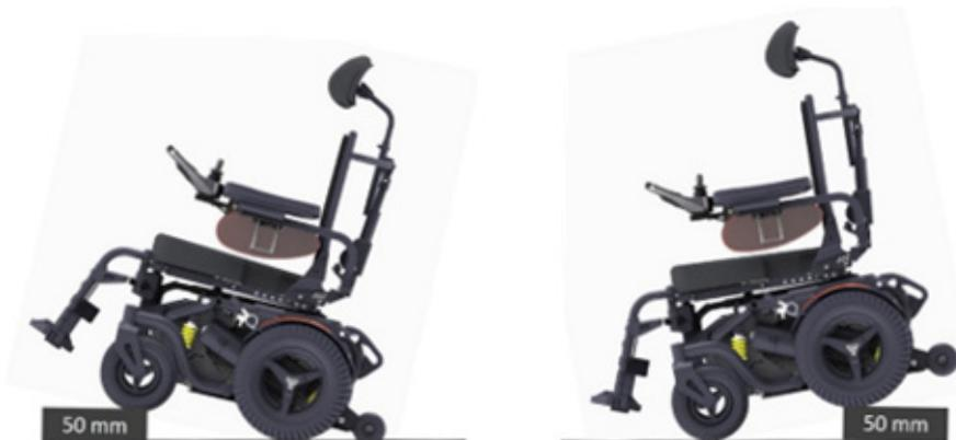
Driving down of a higher surface (like pavement), always be aware of the sudden forward movement of your wheelchair when driving down of it. If your wheelchair has powered seat tilt, you can use the seat tilt for more stability whilst driving of the pavement.
