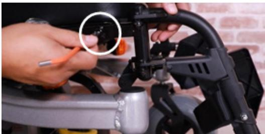
Step 2: Pull out or push in the footrest hanger and find the mounting hole that best fits the user.
