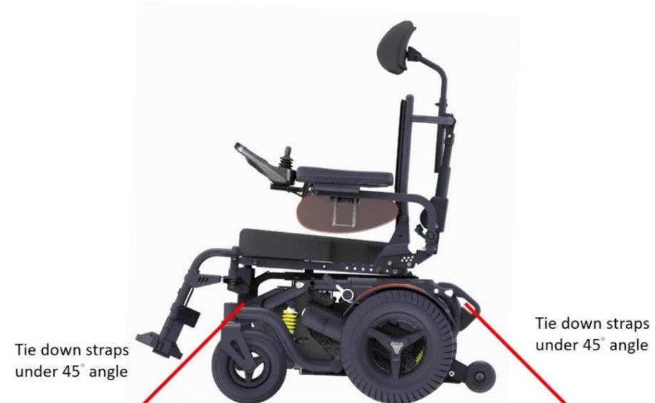
The straps have to be connected to the vehicle at suitable anchor points. Make sure that the tire pressure is at the recommended level so the straps can have maximum effect. Make sure the straps are tightened to maintain optimal security.
