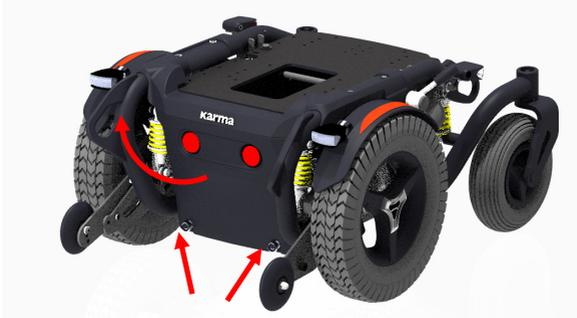
Step 2: Remove the four battery box locking bolts at the front end of the chassis side.
