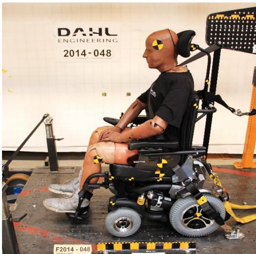
The locking of the wheelchair into the Dahl Docking station makes it much easier to lock down the wheelchair for occupied transportation. It can be used also for wheelchair users who want to drive the car by themselves.
