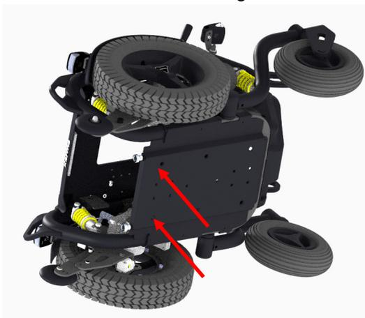
Step 6: Mount the Dahl locking plate by using the 5 high grade Dahl bolts on to the chassis. Secure them with Loctite 222 and tighten them, but not too tight. (16 – 18 Nm).
