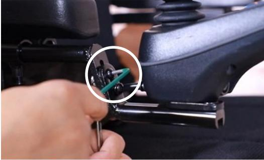
Step 1: Use 3 mm Allen key and 8 mm Open Wrench to loosen up this bolts and nuts.
