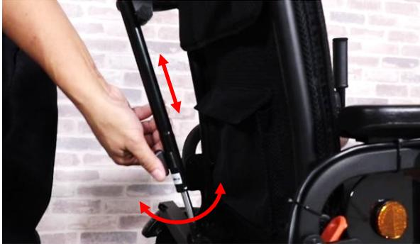
The mechanical adjustable recline backrest uses a stepless telescopic tube with quick release and lock lever action. The manual stepless recline can be set up to 119°.
