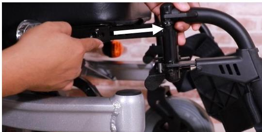
Step 3: Re-tighten the screws. Now the footrests are set into a different position.
