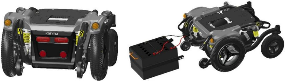
*Position of the maintenance free batteries*
