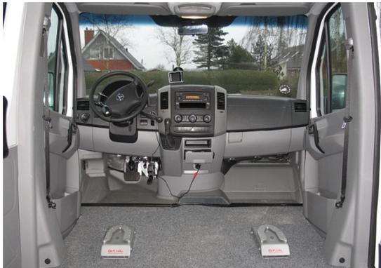
*Dahl docking station mounted on the floor.*
