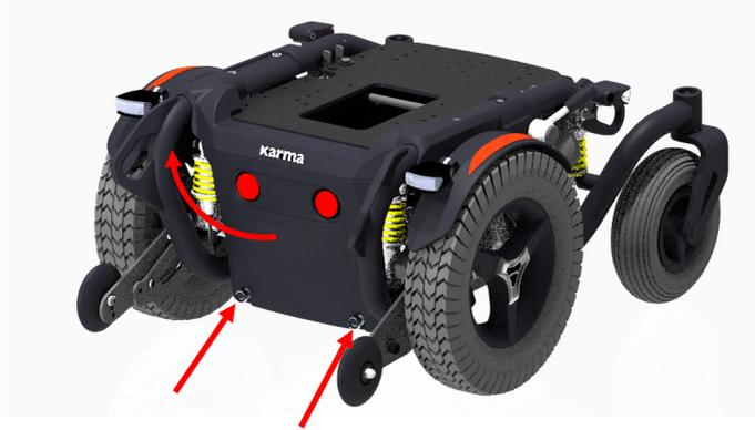
Step 2: Loosen the 4 locking bolts of the battery box.
