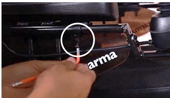
Step 1: Use 5 mm Allen key to loosen up this bolt.
