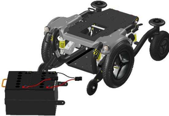
Step 5: Lift the batteries out of the box and disconnect the cables of the poles using a wrench.
