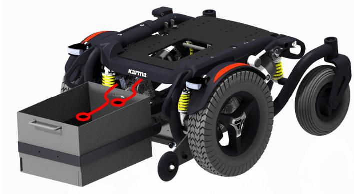
Step 4: Place the mounting plate inside the chassis on the bottom.
