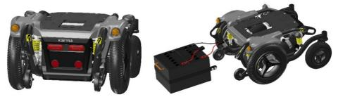
Position of the maintenance free batteries
