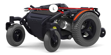
The chassis has very strong and bright LED lights to make sure you can have a safe drive in the dark. The red reflectors in the rear also make you visible for other people as well. The lights fulfill the European requirements. The additional LED indicators give our environment clear information in which direction you want to go.
