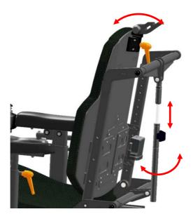
The mechanical adjustable recline backrest uses a stepless telescopic tube with quick release and lock lever action. The manual stepless recline can be set up to 115°.
