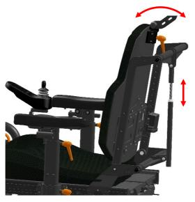
The backrest angle can be set by changing the length of the threaded rod of the backrest tube.
