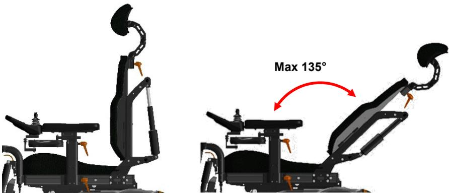
If the reclined backrest position is activated over a certain angle, the driving speed will be reduced. This is to reduce the risk of danger whilst driving at high speed.
