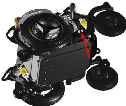
Step 11: Place the front cover back and secure it with the two bolts.
