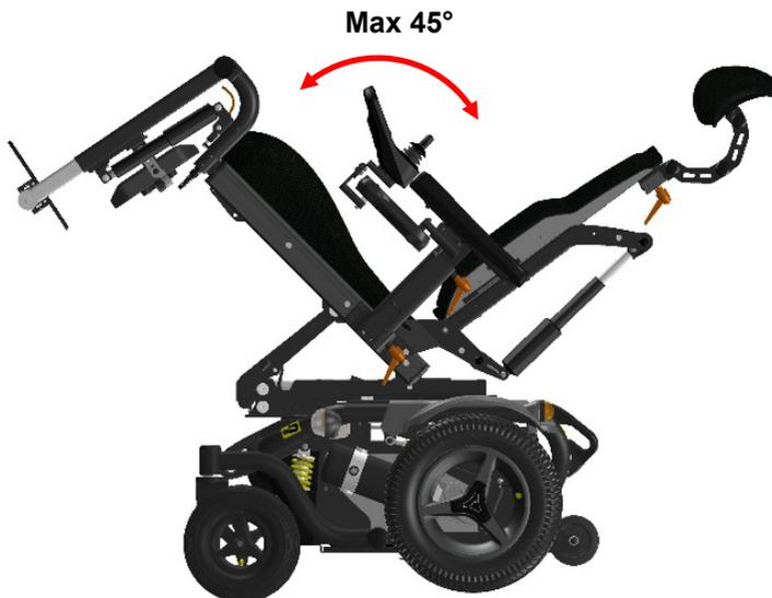
If the tilt is activated over a certain angle, the driving speed will be reduced. This is to reduce the risk of danger whilst driving at high speed.
