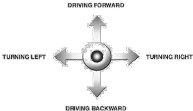
The secondary purpose of the joystick is to navigate through the menu of the wheelchair. By moving the joystick forward or backward you can scroll up or down through the menu, by moving to the right you can enter a sub selection.
