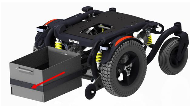
Step 4: Unplug the battery cable connectors.
