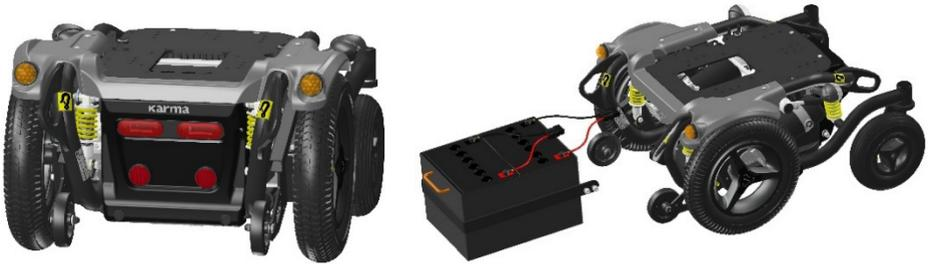
*Position of the maintenance free batteries*
