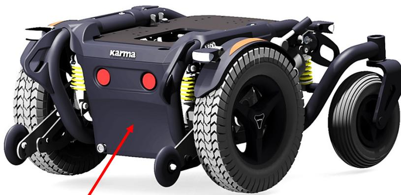
*Position of the battery pole (behind the rear cover)*
