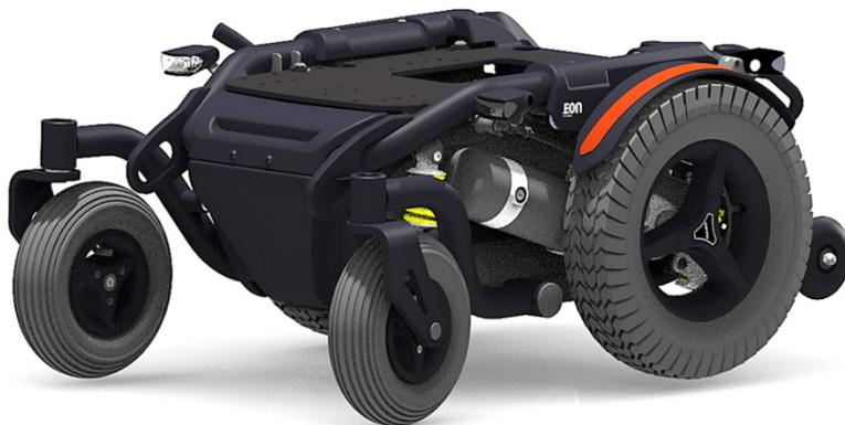
Each of the rear wheels is propelled by a powerful drive motor. These motors also take care for the steering of the wheelchair. With this system it is possible to track straight easily. This makes the wheelchair optimal for outdoor use.
