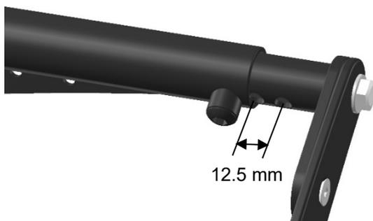
Step 5: Secure the right position by mounting the dome shaped bolts into the designated holes again, then tighten the end bolts to fix that side of the seat.
