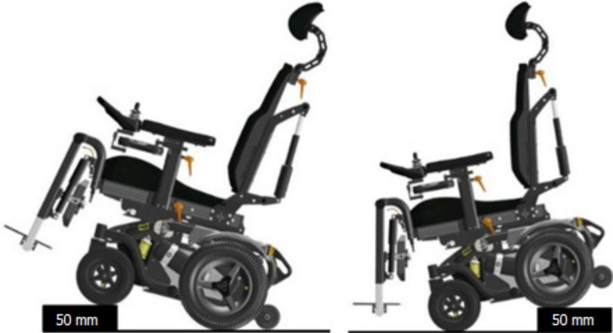
Driving down of a higher surface (like pavement), always be aware of the sudden forward movement of your wheelchair when driving down of it. If your wheelchair has powered seat tilt, you can use the seat tilt for more stability whilst driving of the pavement.
