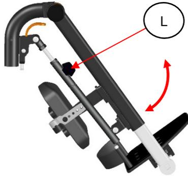
Step 1: To adjust and set the legrest angle, you hold the legrest with one hand and unlock the setting lever (L) with the other hand and push the legrest sideways.
