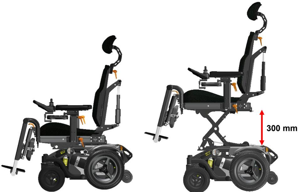
Whilst lifting the seat, the driving speed will always automatically be reduced to gain maximum stability. At high seating position also, the seat tilt will be blocked to gain maximum stability. The seat height can be set to every height position by the user.
