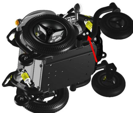
Step 3: Pull the battery box slowly out of the chassis and mind the cables.
