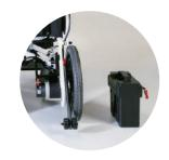
Removable battery 22AH\*2 Battery Capacity-Range 15 km.
