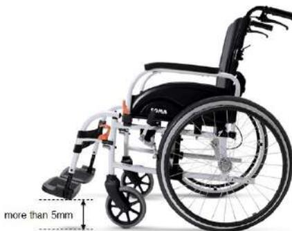
Use 10 mm open wrench and 5 mm Allen Key from KARMA Tool Kit to loosen the bolt and nut at the side of the footrest. Adjust the footrest height and re-tighten the bolt and nut. Now the footrests are set in to a different position. Please make sure the minimum distance between the footplate and the ground should be more than 5 cm.
