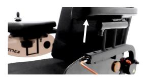
step 2: Adjust the armrest to the proper height and re-tighten the bolts. Now the armrests are set in to a different height position.
