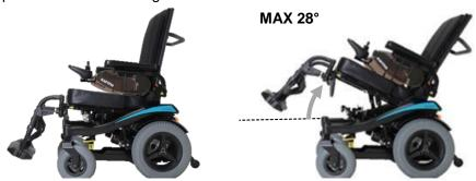
If the tilt is activated over a certain angle, the driving speed will be reduced. This is to reduce the risk of danger whilst driving at high speed.
