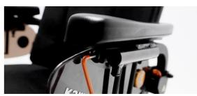
step 1: Use 5mm Allen Key from KARMA Tool Kit to loosen the height adjustment bolts under the armrest pad.
