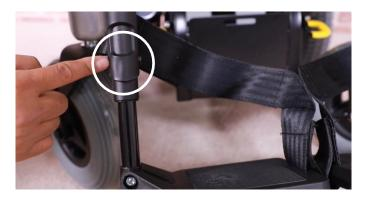
Use 10mm open wrench and 5mm Allen Key from KARMA Tool Kit to loosen the bolt at the side of the footplate and adjust the footplate height and retighten the bolt. Now the footplates are set in to a different position.
