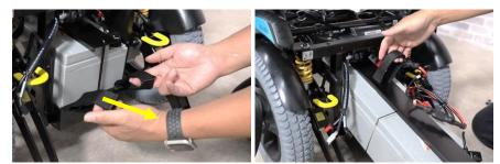
step 9. Use the rear and front strap to pull out the battery plate
