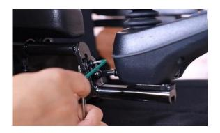
step 1: Use 3mm Allen key and 8mm open wrench to loosen up this bolt. step 2: After confirming the position, re-tighten the screw.
