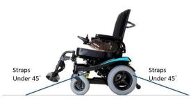
The angle of the straps should be around 45° to the horizontal plane. This is to have maximum effect in vertical and horizontal direction.
