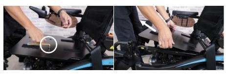
step 2. Use 4mm Allen key to unscrew the bolt connecting the seat plate. When taking off the seat plate, first tilt it up and then pull.
