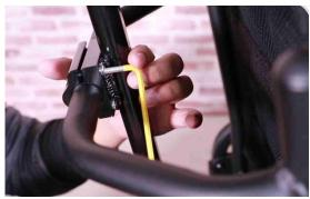
step 1: Use 4mm Allen key to adjust the horizontal position from the bracket connecting the headrest to the frame.
