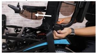
step5. Push the backrest frame to the preferred position. If the frame is tight, use rubber mallet to help.
