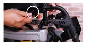
Step1: use 5mm Allen Key included in your KARMA Tool Kit to remove the screws under the seat.
