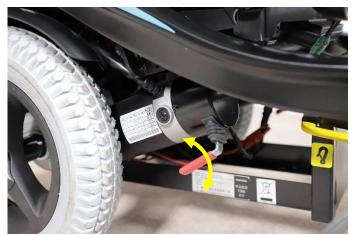
Testing the brake release
