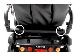
step 1: Use 5mm Allen key to unscrew the screws securing the armrests.
