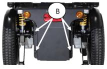
After taking the cover off, the maintenance free battery can be pulled out of the box. Mind the cables! At installing the maintenance free battery, one should pay great attention to make sure the cables are not jammed between the battery and the battery box.
