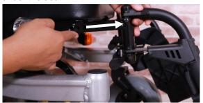
Step2: Pull out or push in the footrest hanger and find the mounting hole that best fitted the user.
