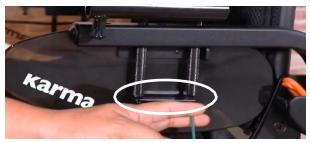
step 1: Use 3mm Allen key to remove two screws shown above.
