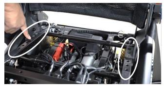
step 4. Use 5mm Allen key to unscrew the bolts connecting the frame.
