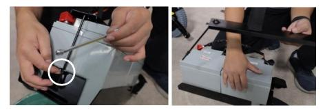
step10. Use 8mm open wrench to loosen up this bolt.
