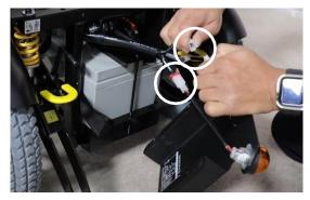
step 8. Disconnect the two light cables
