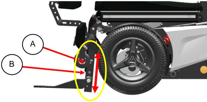
step 1: loosen up the bottom legrest (A) bolt first, using a 5mm Allan key.
