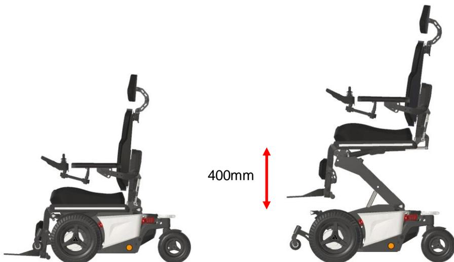
Whilst lifting the seat, the driving speed will automatically reduce to gain maximum stability at all times. At high seating position also the seat tilt will be blocked to gain maximum stability. The seat height can be set to every height position by the user. The maximum seat height is set to 865 mm (seat pan to ground)
