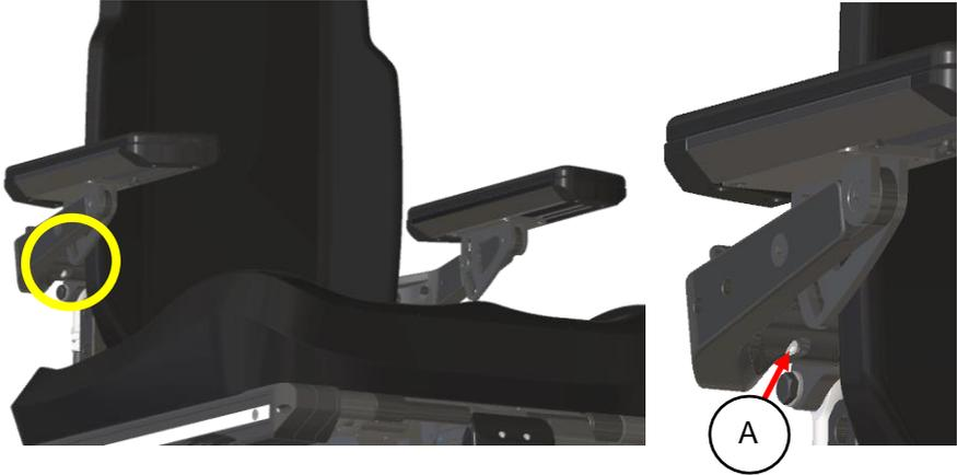
step 1: release the locking bolts (A) on each side of the armrest using an Allan key size 5mm.
