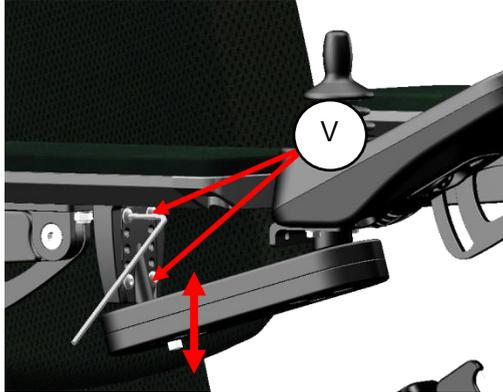
step 1: loosen the 4 bolts (V) using a 3mm Allan key.
