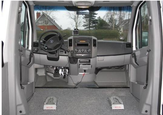
*Dahl docking station mounted on the floor*
