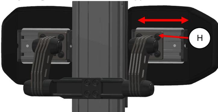
step 1: loosen up the four bolts (H) of the calf support pad, using a 5mm Allan Key.
