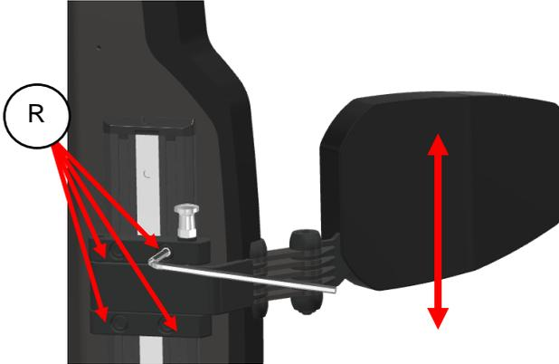
step 1: loosen up the 4 bolts (R) using a 5mm Allan key.
