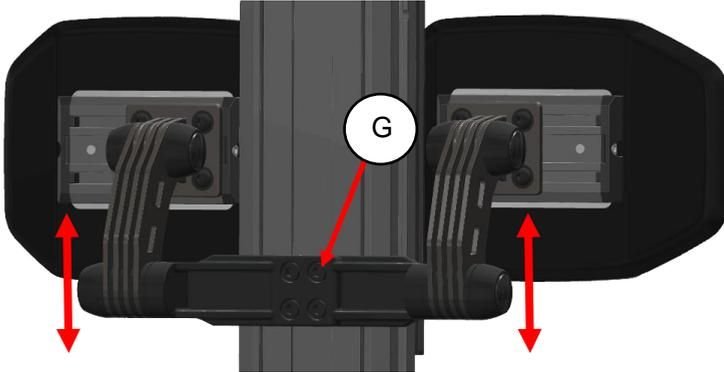
step 1: loosen up the four bolts (G) using a 5mm Allan key, until the calf support starts to slide in the rail.
