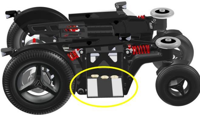
2. Two plastic spacers are to be placed in every battery box on the floor. Best is to fix them with some double sided tape.
