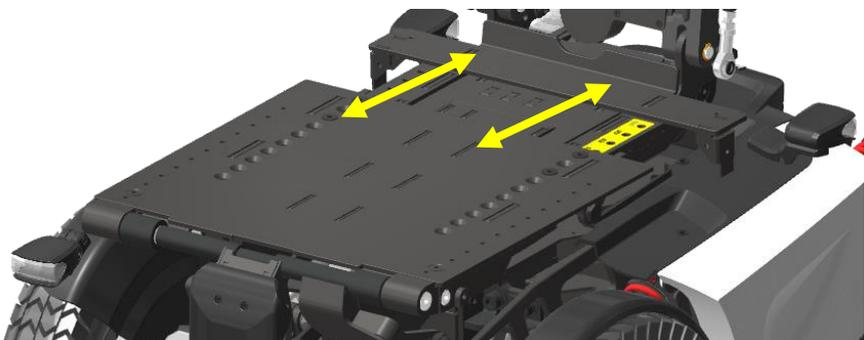
step 6: move the backrest frame backward to increase the seat depth or forwards to reduce the seat depth.
