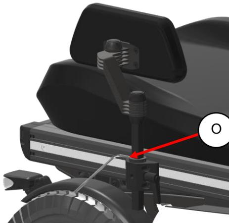
step 2: loosen the bolt (O) of the fixation ring using a 4mm Allan key and reposition this ring against the mounting block as a stopper.
