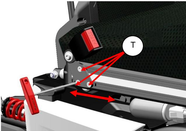
step 1: loosen the 3 bolts (T) using a 4mm Allan key.
