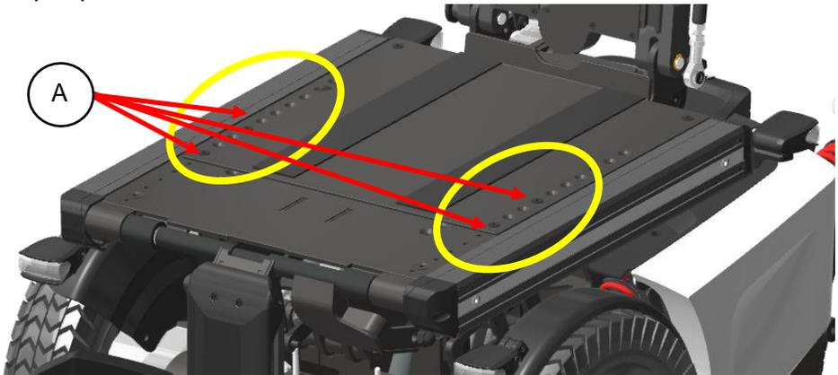
step 2: loosen the top seat panel screws (A) using a 3mm Allan key.
