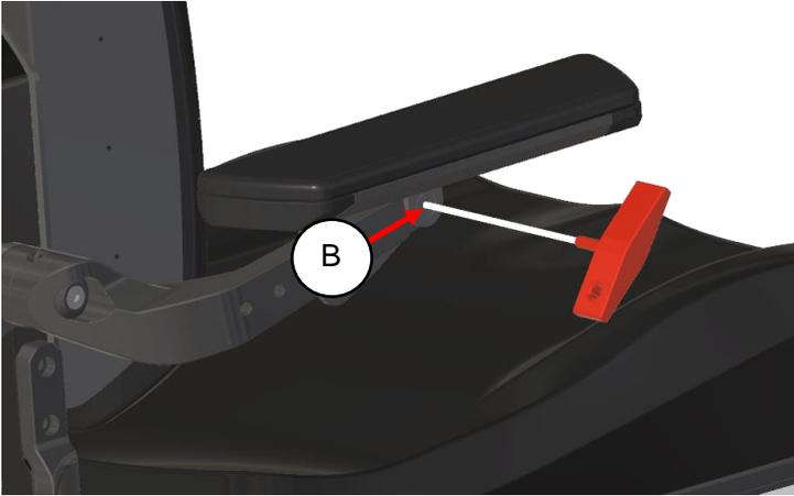
step 1: loosen the front armrest bolt (B) using a 5mm Allen key. Don't take it out, just loosening.
