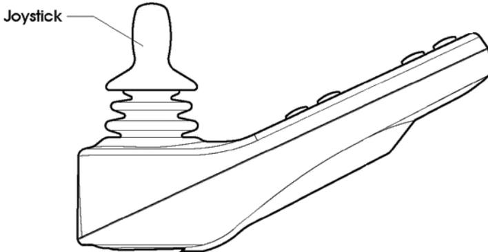
The joystick is primarily used to drive the wheelchair. just push the joystick into the direction you want to drive, and the wheelchair will start to move in that direction.
