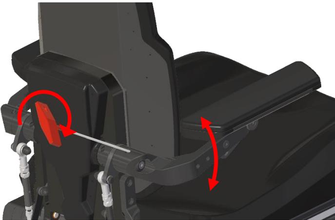
step 2: set the armrest angle by using a 5mm Allan key. By rotating it clockwise the armrest height will increase. By rotating it counterclockwise the armrest height will be reduced.
