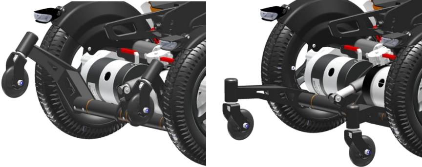
The support wheels prevent the wheelchair tipping over when moving when moving into the vertical position. The support wheels are positioned in front of the drive wheels and are automatically activated by the electronic system.
