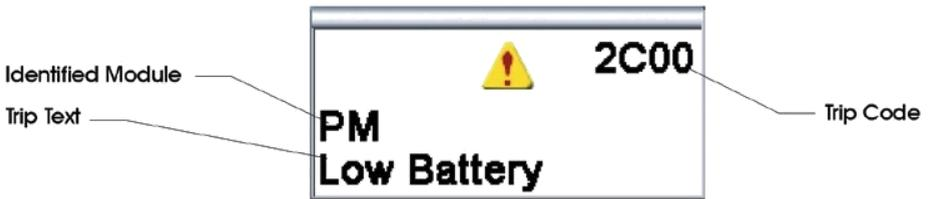
This indicates a system fault, i.e. R-net has detected a problem somewhere in the wheelchair's electrical system.
