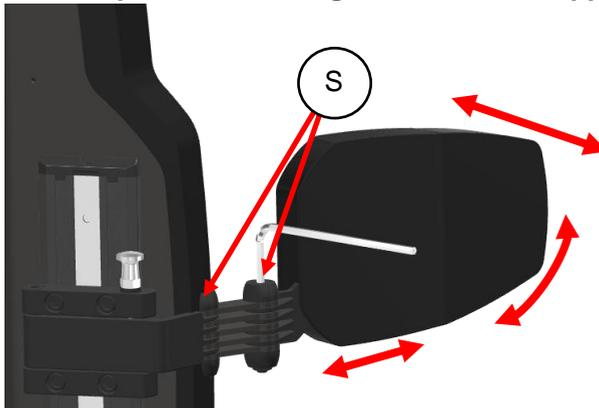
step 1: loosen the 2 bolts (S) of the friction joints.
