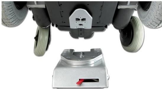
*Docking station and docking plate on chassis*
