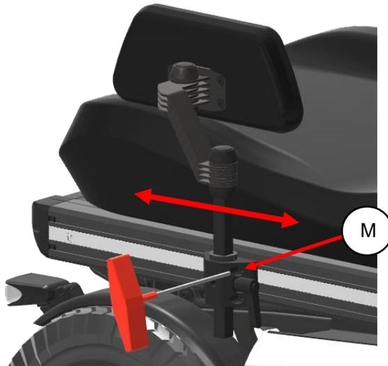
step 1: loosen the four bolts (M) using a 5mm Allan Key.
