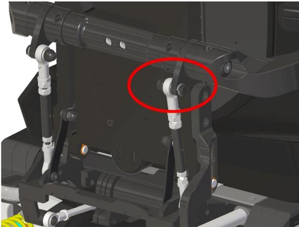
step 3: remove the bolts and detach the parallel bar from the armrest.
