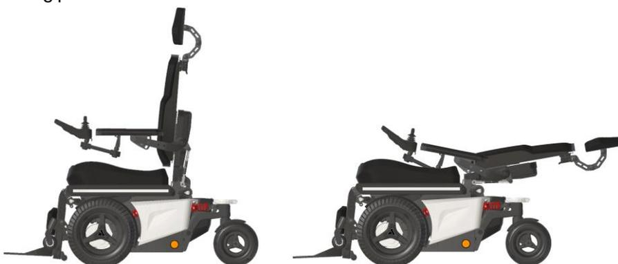
At a reclined backrest position over 135°, the driving speed will be automatically reduced for safety reasons.
