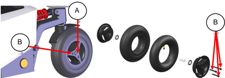
The rear casters should be taken off from the axle by loosening the center bolt (A). The tire can be taken off by loosening the 3 bolts (B) and splitting the rim.
