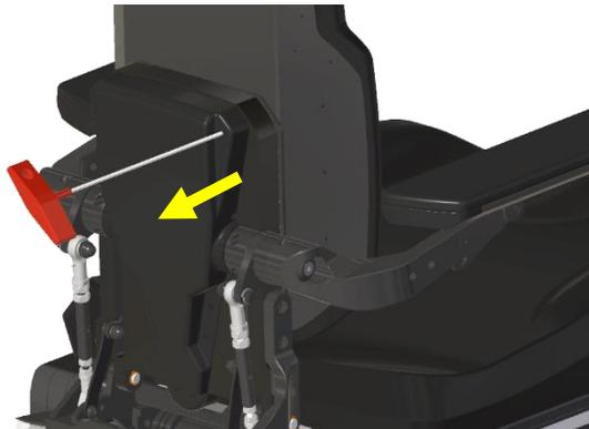
step 1: remove the rear cover of the backrest. To do this you must use a 3mm Allan key to loosen the 6 small screws.
