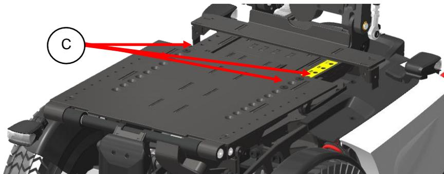
step 5: loosen up the screws (C) of the backrest sliding unit, using an 5mm Allan key.
