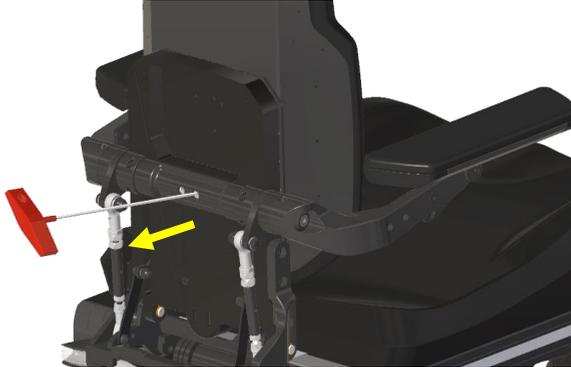
step 2: loosen and remove the two bolts using a 5mm Allan key.
