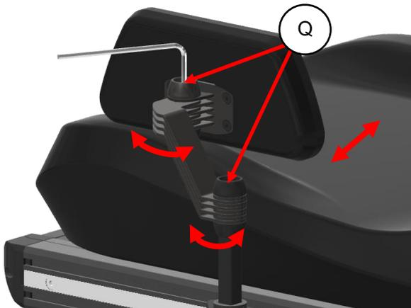
step 5: loosen the 2 friction bolts (Q) so the padding can be moved.
