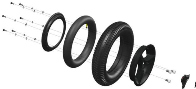
After taking the wheels of the wheelchair, the rim can be split. The tire is then available for repair. The inner tubes of the tires can be repaired according to the description on the tire puncture repair kit that you use. It is however recommended to renew the inner tube at all time when the tube has a puncture.
