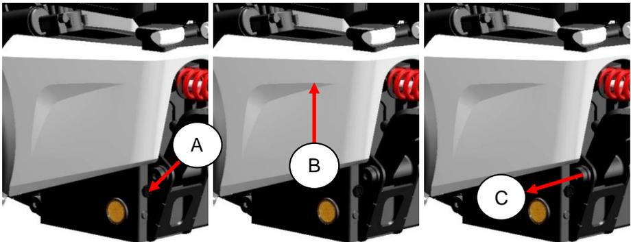
After taking the cover off, the maintenance free battery can be pulled out of the box.
