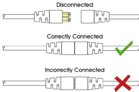
Do not hold or pull on the cable. Always grip the connector when connecting and disconnecting.
