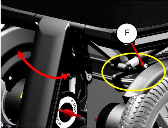
step 1: loosen up the bolt (F) on the telescopic tube of the legrest using a 5mm Allan key. Just open it far enough so you feel it is starting to move.
