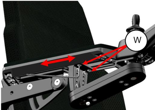
step1: loosen the 2 bolts (W) using a 3m Allan key.
