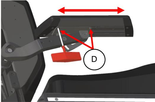
step 1: loosen up the four bolts (D) using a 3mm Allen key.
