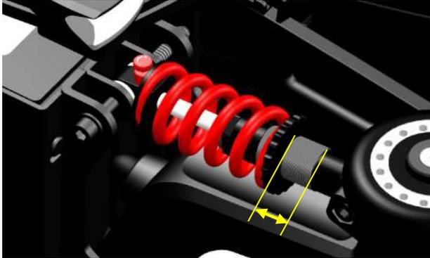
The best way is to measure the distance between the ring and the end of the tread in mm. Make sure that the spring settings in the front are identical. The same for the two rear springs.
