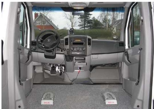
*Dahl docking station mounted on the floor*
