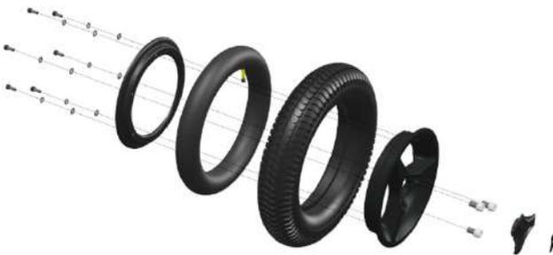
After taking the wheels of the wheelchair, the rim can be split. The tire is then available for repair. The inner tubes of the tires can be repaired according to
