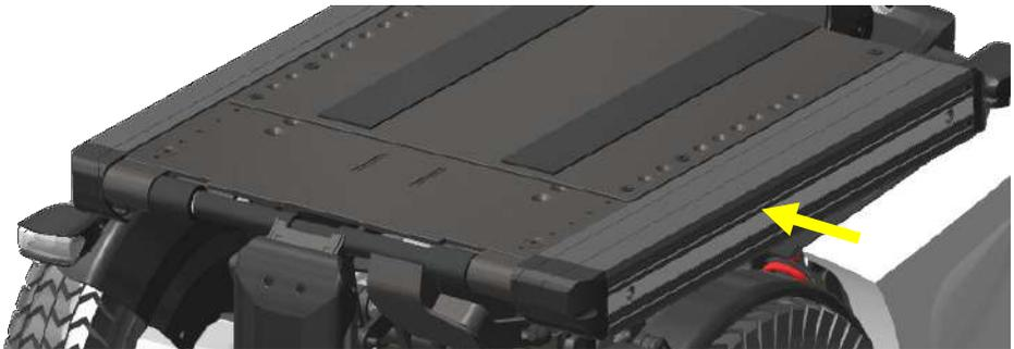
Step 5: Tighten the bolts and place the wider seat cushion on the seat pan.
