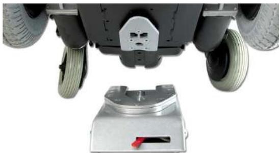
*Docking station and docking plate on chassis*
