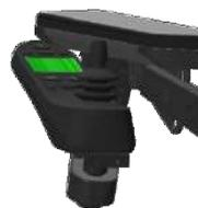
The Evo Lectus Low Rider (EVO-LTS-LR) wheelchair has a side steering control unit, which is either mounted on the left- or right armrest. The joystick module can be mounted on a fixed bracket or on an (optional) swing away mechanism. This system enables you to sit close to a table.
