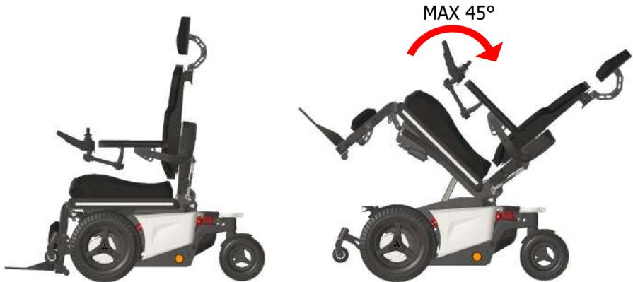
If the tilt is activated over a certain angle, the driving speed will be reduced. This is to reduce the risk of danger whilst driving at high speed.
