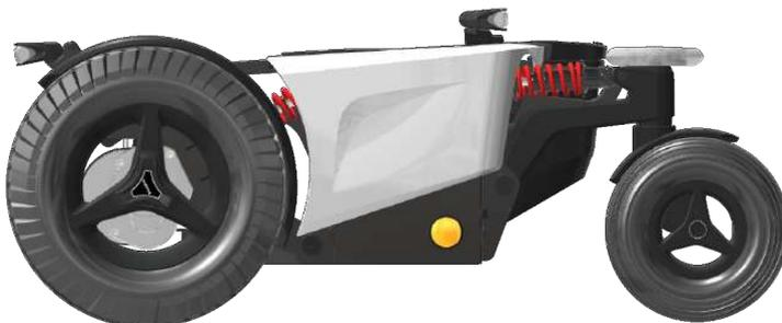
Each of the drive wheels is propelled by a powerful drive motor. These motors also take care of the steering of the wheelchair. With this system, it is possible to turn on the spot. This makes the wheelchair optimal for indoor use.
