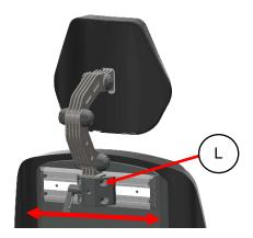
step 1: loosen the 4 bolts (L) using a 5mm Allan key.
