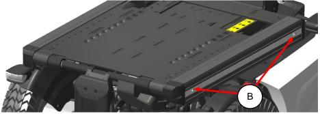
step 4: loosen up the screws (B) of the side rails, using an Allan key size 4mm. And take the side rail away.
