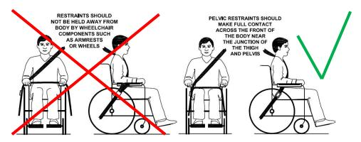
Picture of improper belt fit
