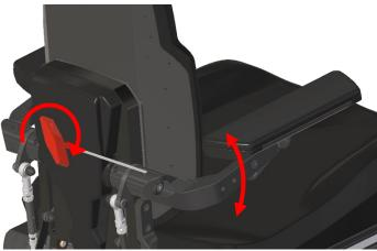
step 2: set the armrest angle by using an 5mm Allan key. By rotating it clockwise the armrest height will increase. By rotating it counterclockwise the armrest height will be reduced.
