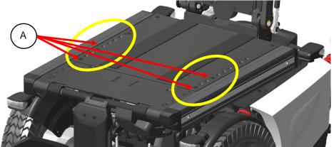
step 2: loosen the top seat panel screws (A) using an 3mm Allan key.
