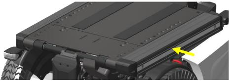
step 4: place the extension rail in to position and place the longer mounting bolt which come with the extension rail.
