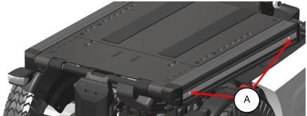
step 2: loosen the screws of the side rail (A) and remove them.
