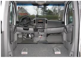
Dahl docking station mounted on the floor
