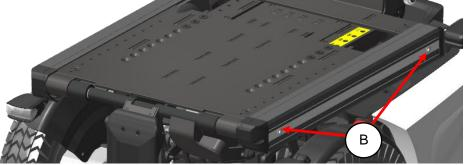
step 8: mount the side rails into position and tighten the bolts (B).
