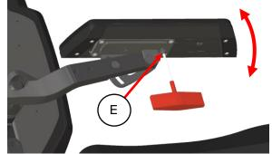
step 1: loosen up nut (E) underneath the armrest pad using a 10mm wrench head.
