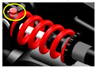
Turning the red knob clockwise will make the movement of the piston going out again faster. This decreases the damping of the spring damper unit. Turning the knob counter clock wise will increase the damping. The right setting will be done by stetting and testing whilst driving. The average setting is halfway. This is set by counting the clicks from the totally left position to the totally right setting. These are 16 clicks. Now set the setting by 8 clicks form the end position.
