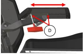
step 1: loosen up the four bolts (D) using a 3mm Allan key. step 2: slide the armrest backward ort forwards into the required position. step 3: tighten the four bolts. The armrest is set.
