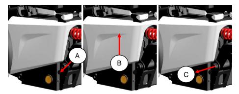
After taking the cover off, the maintenance free battery can be pulled out of the box. Mind the cables!
