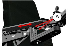
step1: loosen the 2 bolts (W) using a 3m Allan key. step2: move the control in the required depth position. step 3: tighten the bolts again.
