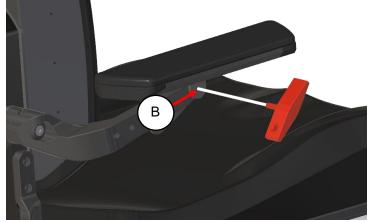
step 1: loosen the front armrest bolt (B) using a 5mm Allan key. Don't take it out, just loosening.
