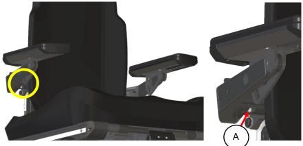
step 1: release the locking bolts (A) on each side of the armrest using an Allan key size 5mm.
