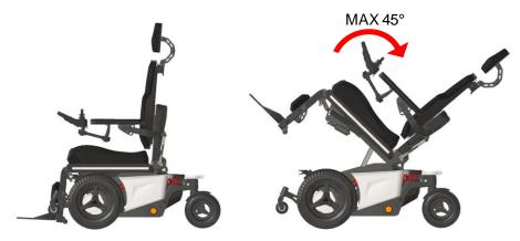
If the tilt is activated over a certain angle, the driving speed will be reduced. This is to reduce the risk of danger whilst driving at high speed.
