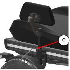
step 2: loosen the bolt (O) of the fixation ring using a 4mm Allan key and reposition this ring against the mounting block as a stopper.
