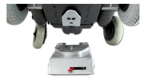
Docking station and docking plate on chassis
