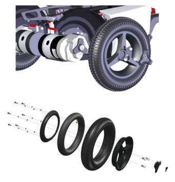
After taking the wheels of the wheelchair, the rim can be split. The tire is then available for repair. The inner tubes of the tires can be repaired according to the description on the tire puncture repair kit that you use. It is however recommended to renew the inner tube at all time when the tube has a puncture.
