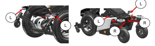
The chassis has very strong and bright LED lights to make sure you can have a safe drive in the dark. The orange reflectors on both sides and the red reflectors on the rear also make you visible for other people as well. The lights fulfill the European requirements. (E marked)
