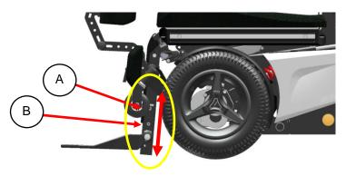
step 1: loosen up the bottom legrest (A) bolt first, using a 5mm Allan key. step 2: slowly loosen up the top end bolt (B). Just enough to feel the footplate is starting to move.
