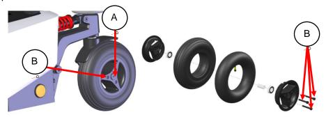
The rear casters should be taken off from the axle by loosening the center bolt (A). The tire can be taken off by loosening the 3 bolts (B) and splitting the rim.
