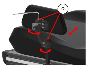
step 5: loosen the 2 friction bolts (Q) so the padding can be moved.
