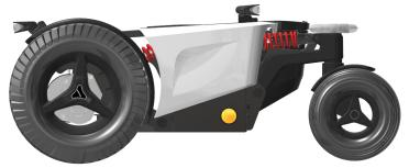
Each of the drive wheels is propelled by a powerful drive motor. These motors also take care for the steering of the wheelchair. With this system it is possible to turn on the spot. This makes the wheelchair optimal for indoor use.
