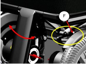
step 1: loosen up the bolt (F) on the telescopic tube of the legrest using a 5mm Allan key. Just open it far enough so you feel it is starting to move.
