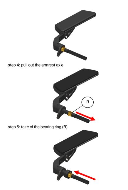
step 6: add or remove the spacer of the axle and put the bearing back.
