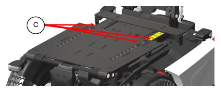
step 5: loosen up the screws (C) of the backrest sliding unit, using an 5mm Allan key.
