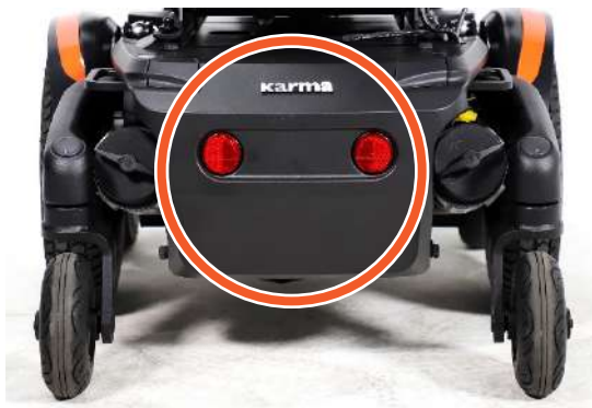
Position of the rear maintenance-free batteries
