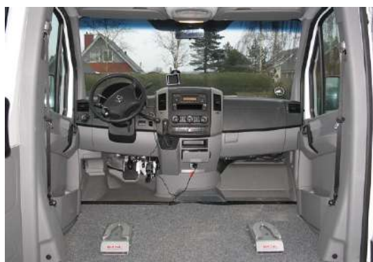
Dahl Docking Station™ mounted on the floor
