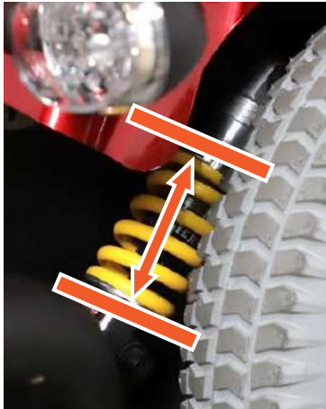
Measure spring setting between left and right sides
