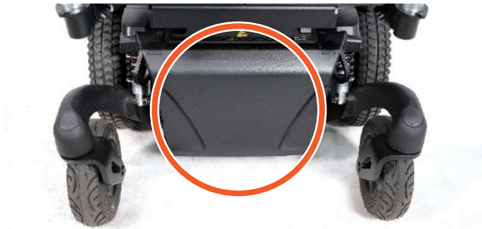
Position of the front maintenance-free batteries
