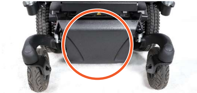
Front battery box
