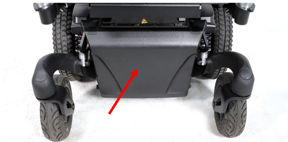
Position of the battery pole (behind the black cover)
