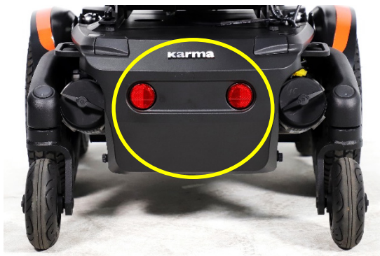
Position of the rear battery box
