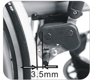
4.3.2.5 To re-adjust, loosen the screw and set the appropriate gap. Then re-tighten the screw. (See the photo on the right)
