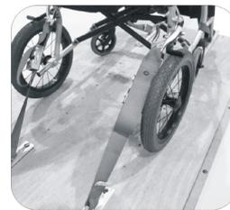
Fitting the rear restraint
