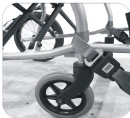
Fitting the front restraint
