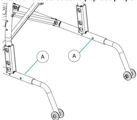
To turn the anti-tippers into the inactive position, rotate the anti-tippers by pressing the release buttons (**A**) and turning them up. Ensure the release buttons pop out again into place (**B**).
