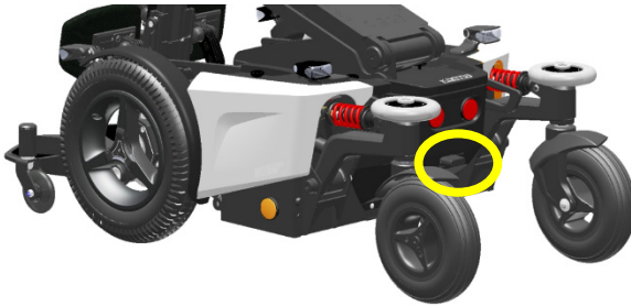
Position of main fuse
