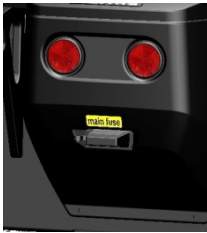
Position of the main fuse
