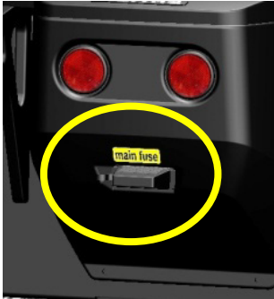
Place of the main fuse
