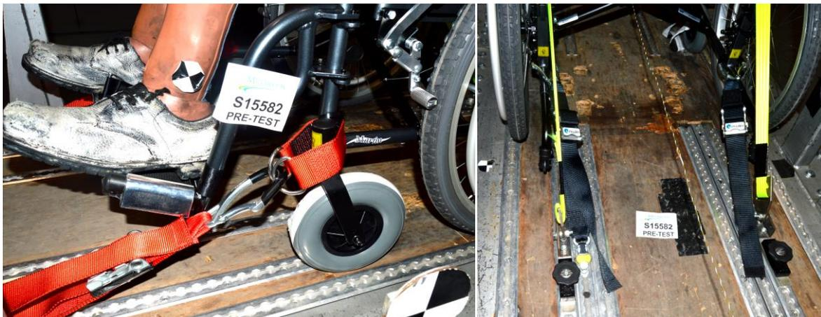
Fitting the Front Restraint
